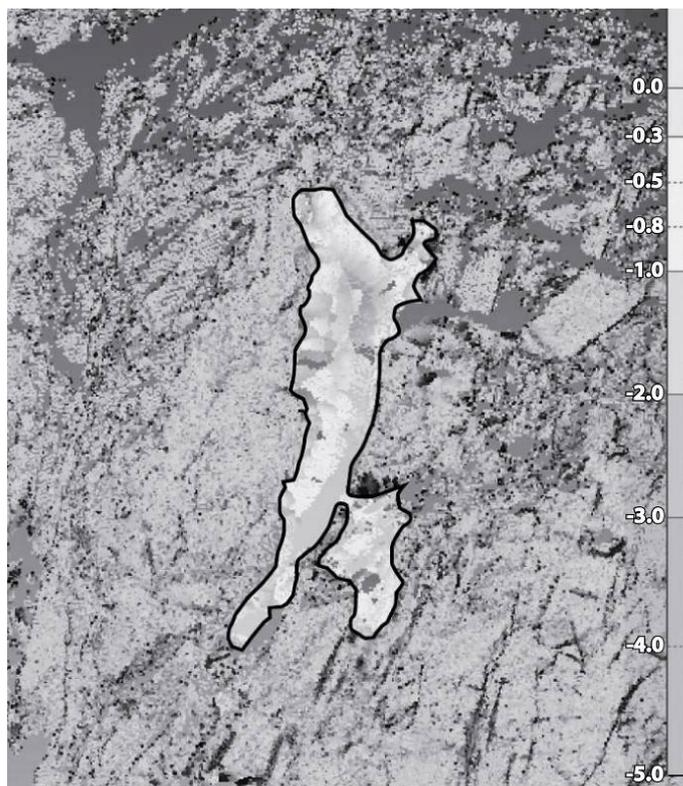
Figure 1. Detail of the map of the errors resulting from the comparison of the 3D models of July 2006 and July 2007, West face of the Grand Flambeau (3561 m a.s.l.). The notch is 15 m high and 4 m large, with a collapsed volume of 57 m<sup>3</sup>. Scale of grey on the right indicates changes in depth (in meters).
